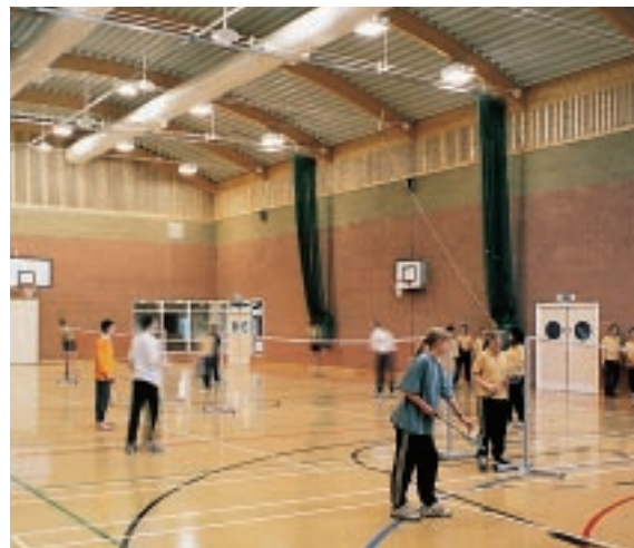
Sports hall structure, lights and division netting must be aligned between badminton courts.
